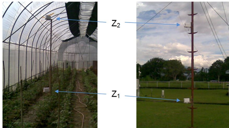
Figure 3-4. Data logger set-up for Bowen ratio measurement.
